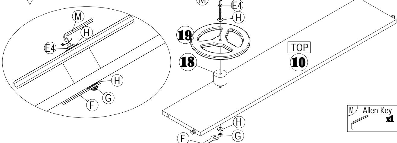
Using the Spanner (F) and Allen Key (M), ensure that the Bolt (E4) and Locking Nut (G) are securely fixed and that the wheel can still turn freely.
