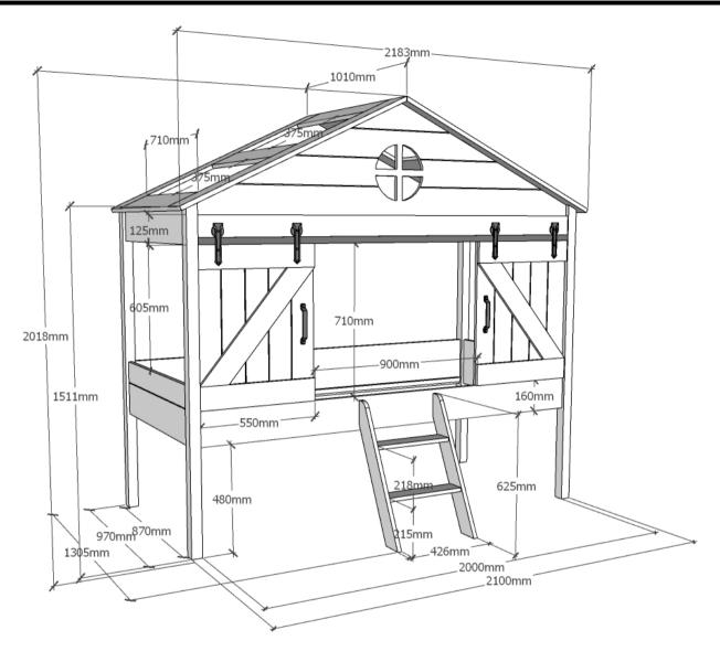
L:2183mm x H:2018mm x D:1010mm (1322mm) innersize:900x2000mm
