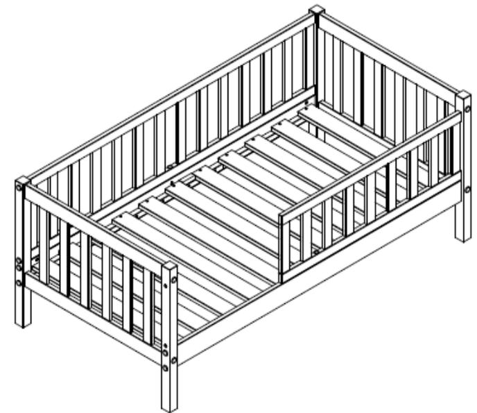
L: 1480mm H: 600mm D: 758mm INNERSIZE 1400x700mm
