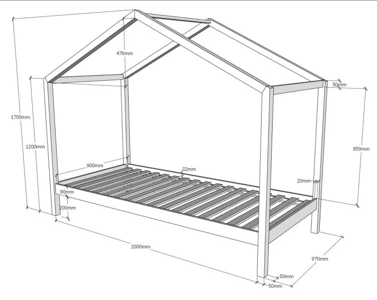
L:2100mm H:1700mm D:970mm innersize 900x2000mm
