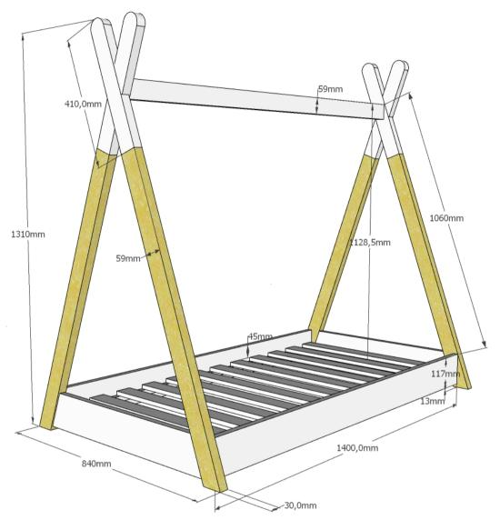
L:1460mm H:1310mm D:840mm innersize 700x1400mm
