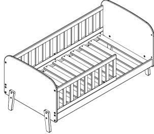
L: 1474mm H: 683mm D: 770mm INNERSIZE 1400x700mm
